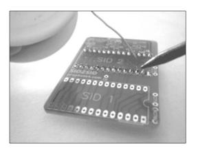
Attach the socket by soldering the pins on the bottom side.
