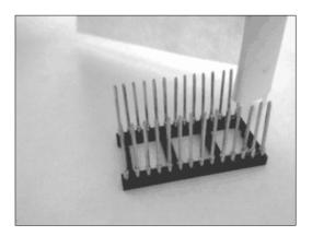
The SID2SID holes are 1.0 mm which is compatible with most sockets on the market. If you experience problems when inserting the long legged socket into the SID2SID holes you might need to sandpaper the legs a little first.
