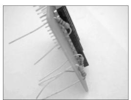
Insert the resistors from the top down just like the sockets, solder them and cut the legs.
