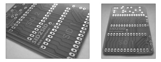
The SID2SID Printed Circuit Board is a single sided board with copper layers and silk screen text on one side only. The idea is to place the components on the opposite side and solder them on the printed side making soldering a lot easier. Installation is made with printed side facing down.
