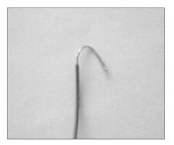
A good advice is to make a curve out of the end of the wire and thereafter hook it onto the pin from behind. Solder it and trim it so that it doesn't short the other pins.
