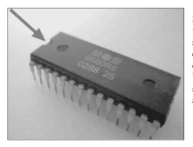
Start by installing the socket for SID #2. Insert it from the top side (the one with no text). Make sure the cavity on the socket is facing the same direction as the cavity on the white circuit outline on the opposite side of the SID2SID. When inserting the SID chips later on this very same cavity on the chips is your guide to correct alignment.
