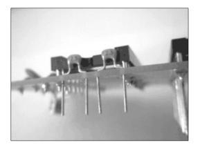
Image shows 22000 pF (22 nF) capacitors for 8580 SID #2 inserted and ready to be soldered. Alignment of the legs is unimportant as these resistors do not have fixed plus and minus poles.
