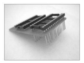
Solder the SID #1 socket just like the one for SID #2. It's a little trickier due to its long legs being in the way for the soldering iron. Be patient.
