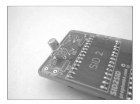
Even though space is an issue you need to make some room for the transistor to move.
