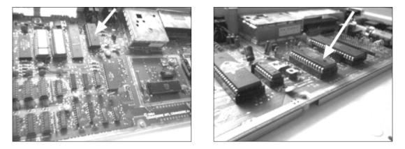
There are three places to find the SID circuit on C64 motherboards. The most common are shown in the pictures above. To the left is the 6581. Right beside the RF modulator (TV output) and to the right is the 8580, placed right below the RF modulator.
