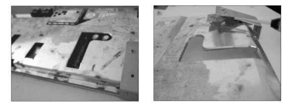
Most of the Commodore computers have some sort of cover on top of the motherboard whether it is cardboard paper or metal. In case your C64 has a metal cover you need to take some action to make room for the SID2SID. It will not fit with the cover back on.
