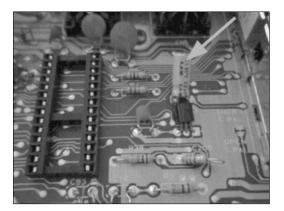
If you have a C64 with the 6581 SID there's only one obstacle, the large capacitor to the right of the socket (as seen in the middle of the image above). You can bend it a little, it won't go all the way down but it's nothing to worry about.
