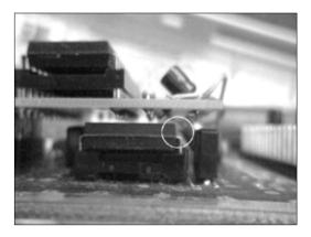
The image above visualizes the problem. At the bottom you see the CIA timer B chip in a socket (which brings the timer circuit even closer to the transistor making the problem worse) and the transistor nearly touching the legs. Metal against metal means a nasty short circuit. (If you can't see it, look inside the white circle. The transistor is slightly out of focus.) Cover the transistor with a piece of tape and bend it carefully away from the timer chip. Keep an extra eye on this!
