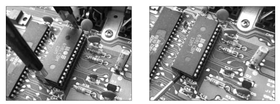
If you use an IC extractor tool you need to pull the chip straight up or the pins might bend. Many people find it easier to use a screwdriver: Insert it gently under one side of the SID and jerk the circuit upwards. Alternate sides evenly. You need to put one finger on the black top on the opposite side and push back a little to keep it leveled (don't touch the pins though). Watch out for electrostatic discharges, wiring your wrist to ground is recommended.
