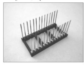
This socket is for SID #1. It's an open frame socket, 600 mil wide. (15.24 mm / 0.6 inches)
