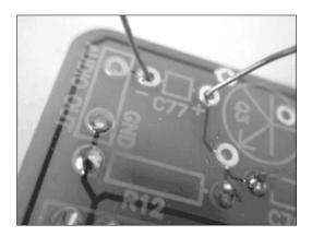
C77 (10 uF) does however have a fixed plus and minus pole so make sure it's inserted correctly.
