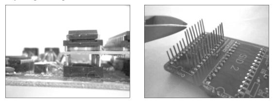
The SID2SID is a very thin board yet sockets and SIDs on top of that bring additional height. By cutting the legs of the long SID #1 socket you can adjust that height. In fact, if your computer has the 8580 motherboard you will find that the keyboard and top cover won't come back on unless the SID2SID is lowered. For 6581 motherboards it's not that big a deal but it is still advisable to lower the SID2SID just a little bit.
