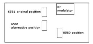
The third place to find 6581s is in the center of the motherboard. This is true for very few older boards. Read the printing on the circuits to make sure it really is a SID before you proceed.
