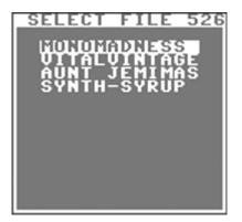
The file operations for the floppy drive make use of the operating system's basic disk functionality. There are no delete-functions and no replace-and-save options built in. If you try to save the file onto disk using an already existing name the save is interrupted and the drive light flashes.
