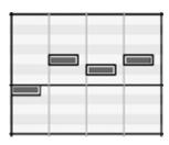
Therefore, when working with an external sequencer, shorten the length of notes so that a note off doesn't get too close to the next note on (right image).
