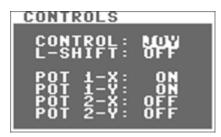
The second option blocks the potentiometers unless the **LEFT SHIFT** key is depressed. Why? Well, as you will notice, potentiometers can be a bit 'shaky' switching values periodically. It's not so much of a problem when turning the VCF frequency or LFO amount but causes unintentional tweaks in case you select the wrong parameter by accident. The L-Shift option only passes through your pot movements
